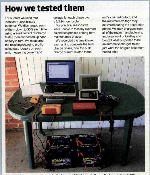
We tested the chargers using four identical Numax 105Ah leisure batteries discharged down to 30%
